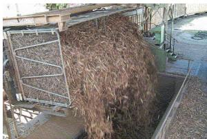
In some installations, the weighbridge and tip are combined, while in other sites, these can be several hundred metres apart. The automatic control of these two devices is unique to each installation. Control strategies have been developed for a number of configurations which utilise PLCs for the field I/O control
