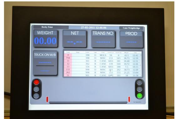
Vehicles fitted with automatic identification would usually not require driver entry in addition to providing driver access, the display provides a dynamic mimic of the weighbridge operation, illustrating weighing sequence stage, advisory, error messages and full details of the pending transaction. With this information now available to the driver in real time, they are kept fully informed at all stages of the weighing operation.
