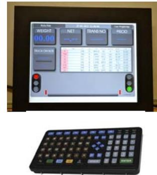
Vehicles fitted with automatic identification would usually not require driver entry. In addition to providing driver access, the display provides a dynamic mimic of the weighbridge operation. Illustrating weighing sequence stage, advisory, error messages
