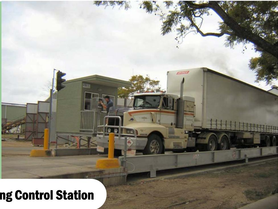
The AWCS R3 is the third generation of this product and incorporates all the features of the previous releases, as well as building on experiences gained from these earlier releases. It has been designed to provide a fully automated weighbridge operation without manning. This is achieved by the extensive use of a dynamic web based mimic.
